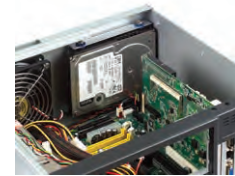
Shock-resistant drive bay for holding an internal 3.5" HDD
