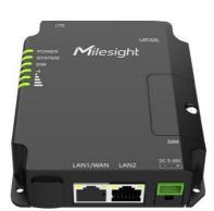
UR32L is a cost-effective industrial cellular router with embedded intelligent features that are designed for multifarious M2M/IoT applications. Global WCDMA and 4G LTE carrier supported make this drop-in connectivity a great help for operators in maximizing uptime. UR32L also has 2 fast Ethernet ports, which delivers users an uninterrupted internet access.
