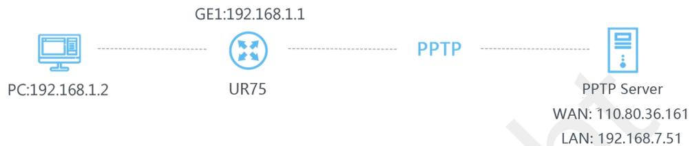
Configure the UR75 as PPTP client to connect to a PPTP server in order to have data transferred securely. Refer to the following topological graph.
